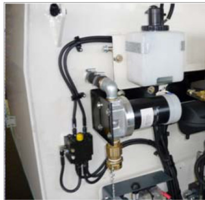
Mounting position of a diesel filling pump
